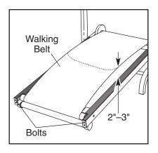
turn both rear roller bolts counterclockwise 1/4 of a turn. When the tension of the walking belt is correct, you should be able to lift each edge of the walking belt 2 to 3 inches. Walk on the treadmill for a few minutes. Repeat until the walking belt is properly tightened. Be careful to keep the walking belt centered.
